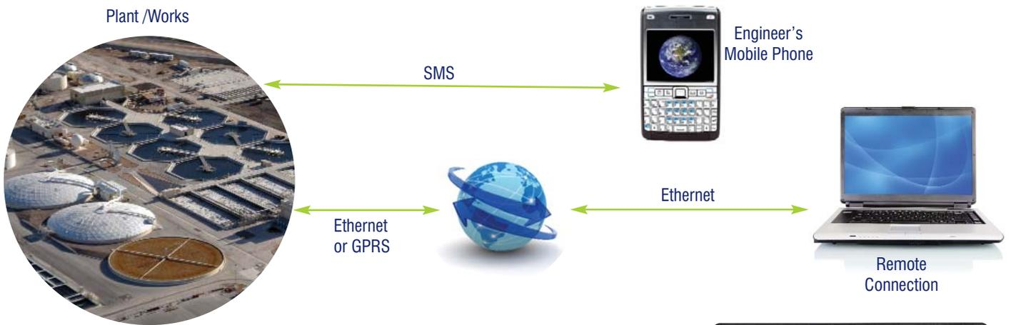
Remote monitoring, control and programming of devices can reduce service visits required and allow first class customer service to be provided to end customers. It minimises downtime, maximises productivity and reduces servicing costs by allowing the possibility of fault diagnosis without visiting site.
